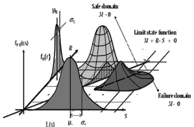
Figure 1. Failure probability determination
