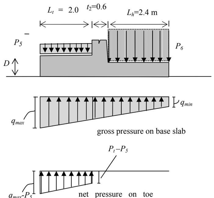
Figure 7. Pressure distribution on toe slab
