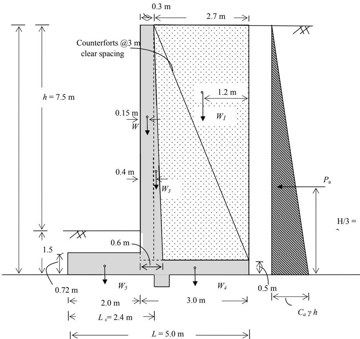
Figure 3. Typical Cross Section of the Counterfort Retaining Wall (Pillai and Menon, 2009)
