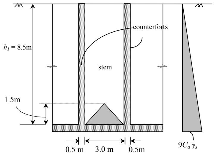
Figure 5. Loading considerations for simplified analysis of stem
