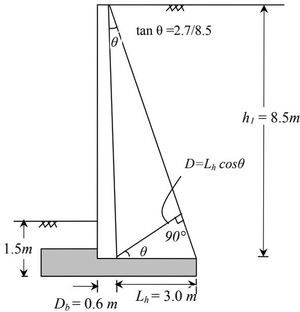
Figure 8. Depth consideration for analysis of counterfort
