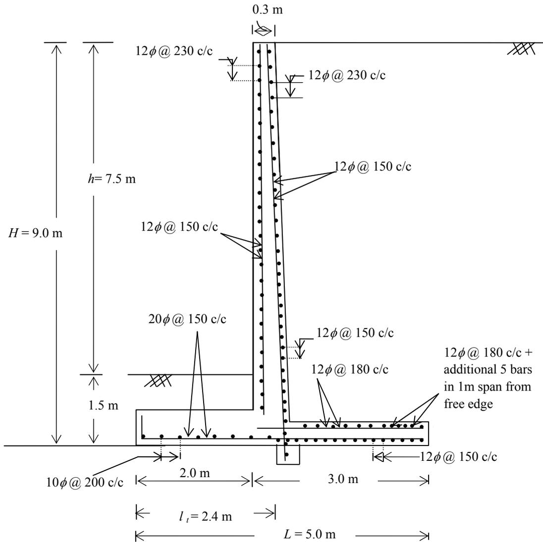
Figure 4. Reinforcement details on stem, toe slab and heel slab.
