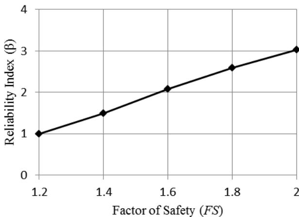
Figure 9. Variation of  $FS - \beta$  for sliding mode of failure
