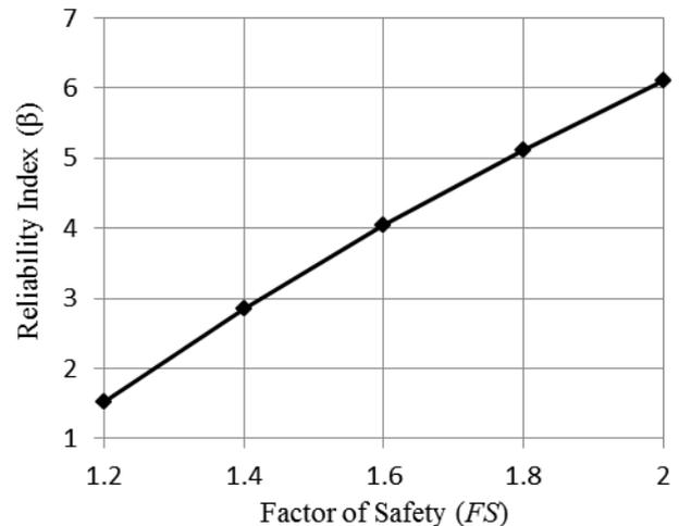
Figure 10. Variation of  $FS - \beta$  for overturning mode of failure.
