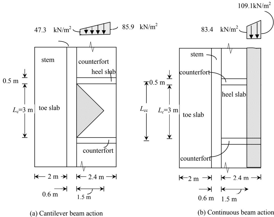
Figure 6. Loading considerations for simplified analysis of heel slab.
