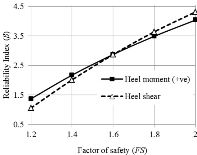
Figure 11. Variation of  $FS - \beta$  for moment and shear mode of failure for heel slab
