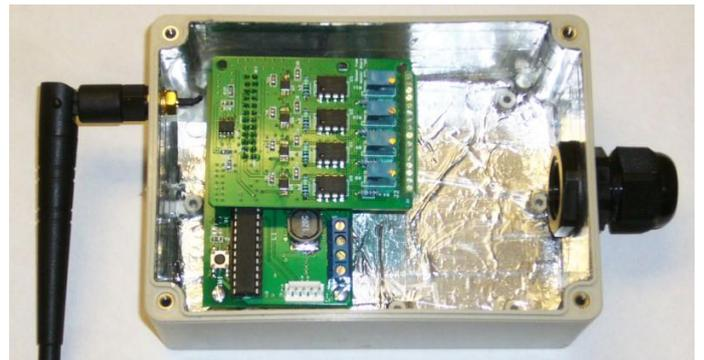
Figure 3: Weather-proof wireless sensor node with lid off
