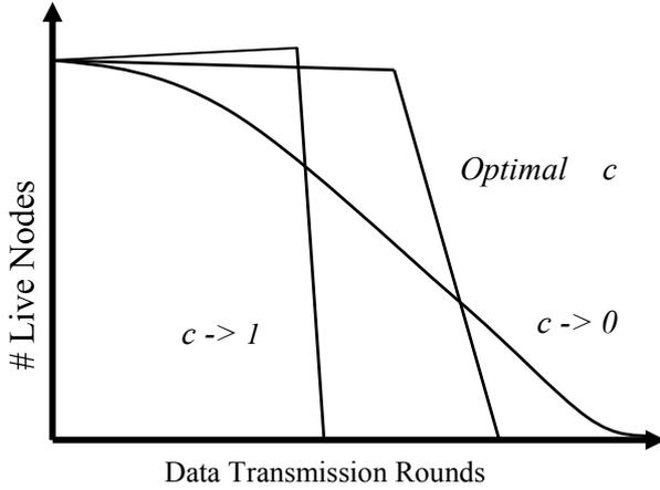
Figure 4: Lifetime of WSN with respect to the change of  $c$
