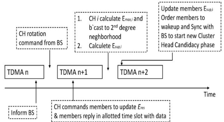
Figure 3: CH Rotation process once it triggered by any CH
