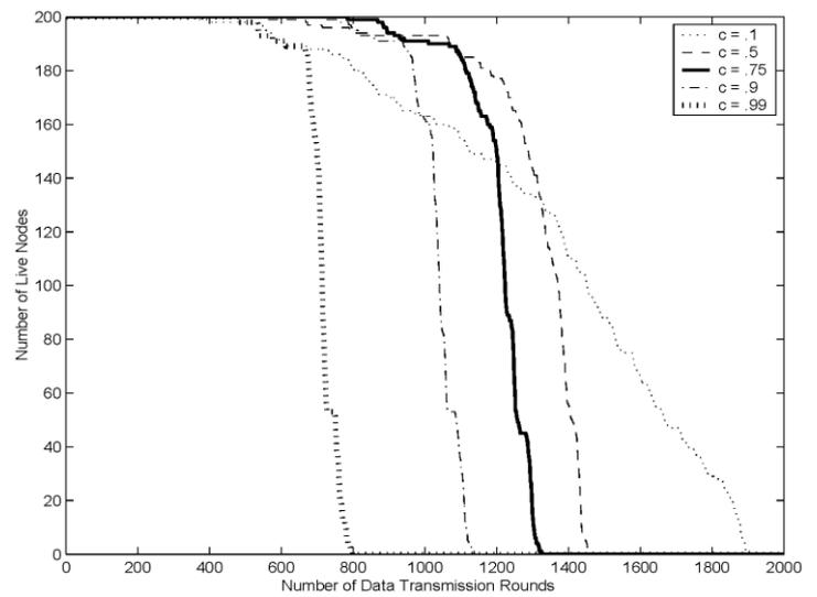
Figure 8. Lifetime Curves of a WSN for different  $c$
