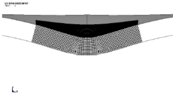
**Figure 8. 50 mm thick PCRC panel with 100% aramid lacing**
