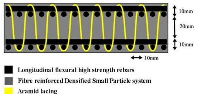
**Figure 3. Principle of 50 mm CRC deck improved for close-in detonation**
