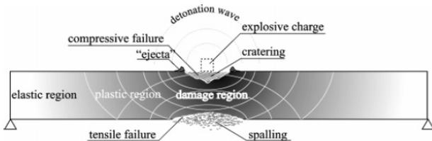
**Figure 1. Contact detonation on a concrete plate, regions of different stress states and failure situations**
