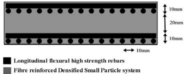
**Figure 2. Principle of a 50mm CRC deck**
