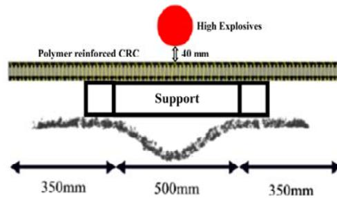
**Figure 4.** Experimental setup for 50x1200x1200 panel – 3.5kg of PETN HE
